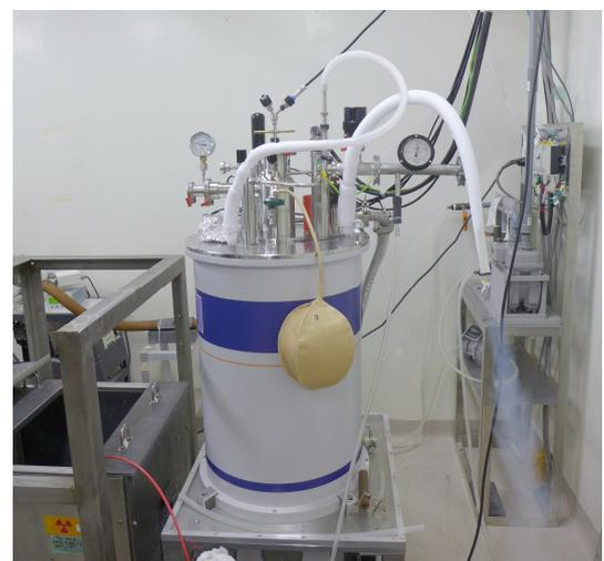
図3: 6T超伝導磁石(Oxford Instruments)
