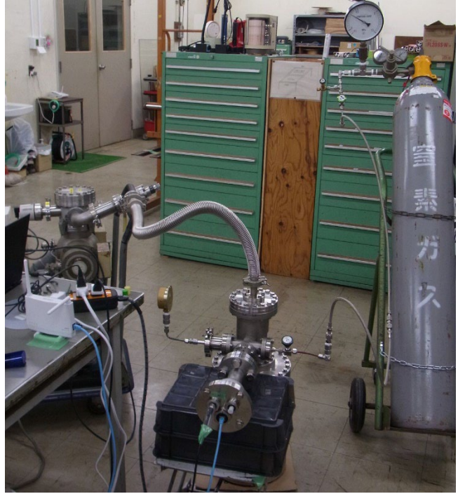
Fig. 1. Offline tests of the vacuum gauge.
