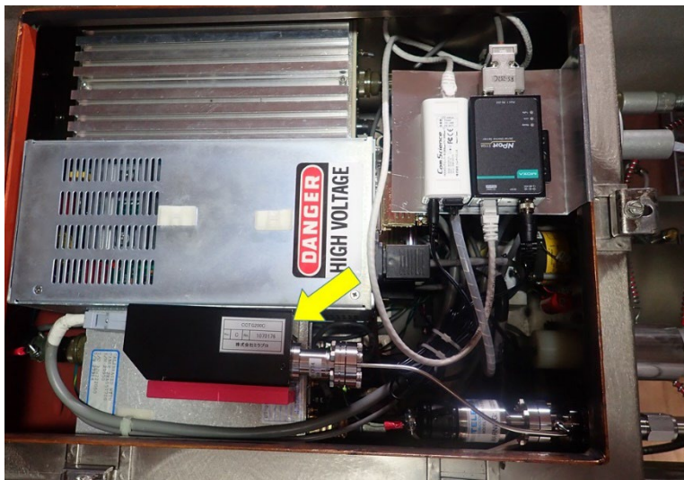
Fig. 2. Inside the shielded terminal box with the connected new vacuum gauge (indicated by the yellow arrow).
