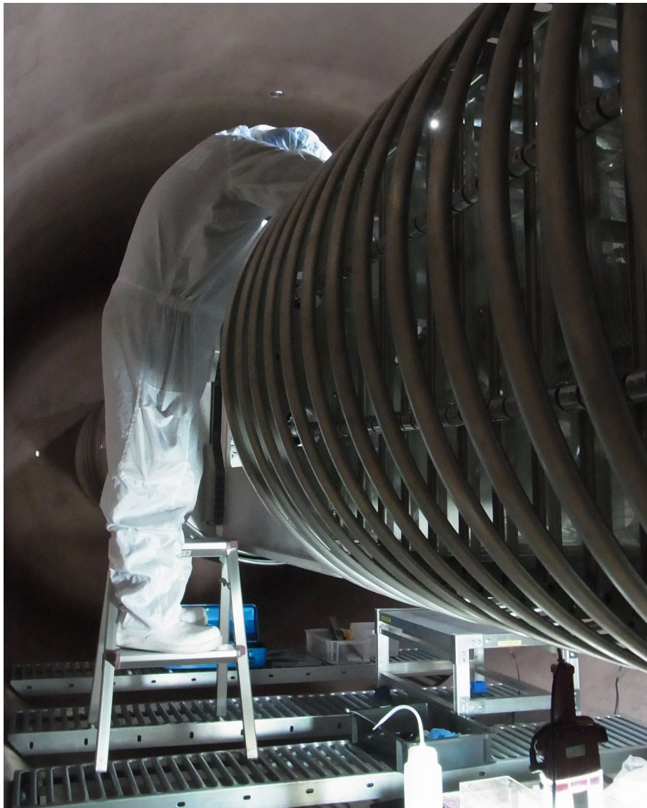
An engineer of UTTAC working for maintenance and upgrading of the 6MV tandem accelerator.
