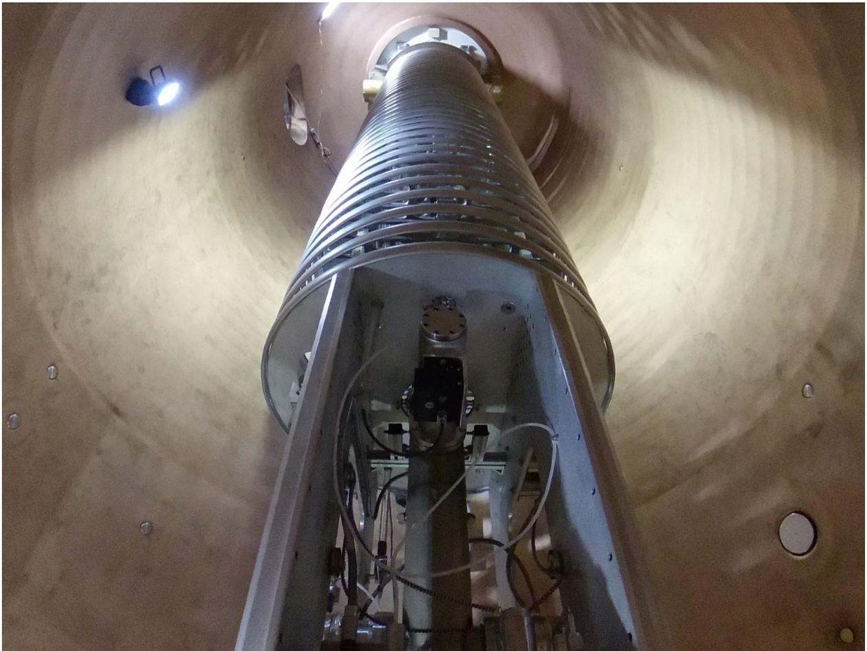
*Acceleration tube of the UTTAC 6MV tandem accelerator, viewed down from the central terminal to the high-energy end.*
