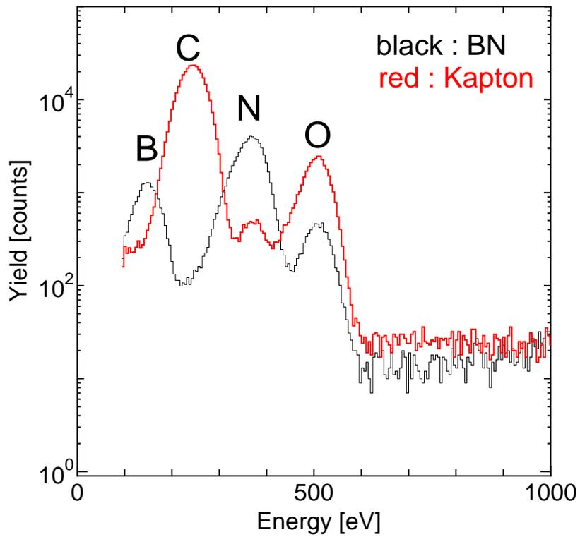
Fig. 2. X-ray energy spectra obtained by SDD with a thin silicon nitride ( $\text{Si}_3\text{N}_4$ ) window.
