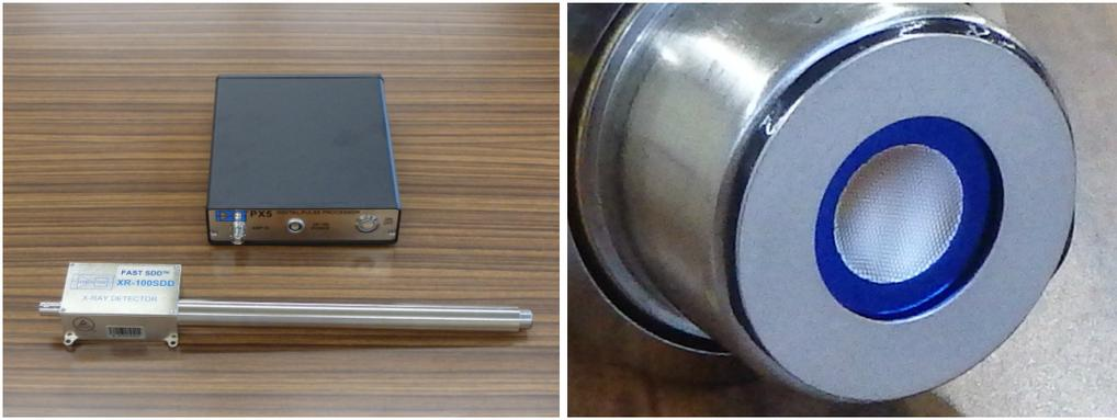
Fig. 1. Photographs of the silicon drift detector XR-100FastSDD with digital pulse processor (Amptek Inc., US) (left). An entrance window is made of silicon nitride ( $\text{Si}_3\text{N}_4$ ) with a thickness of 40 nm for observing characteristic X-rays from light elements (right).
