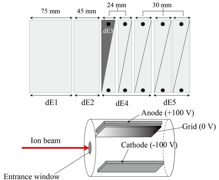
Fig. 1. Five-anode type  $\Delta E$ -E detector.
