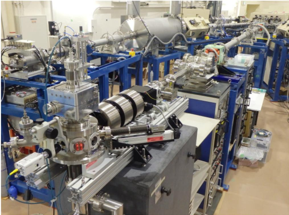
Fig. 1. Photograph of the ion microbeam line at UTTAC.
