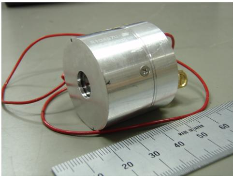
Fig. 1. The high speed HPD (HAMAMATSU R10467U-06).
